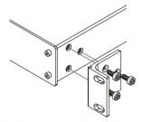
2. Place the ears of the machine against the rack rails, and insert the proper screws (not provided) through each of the four holes in the rack ears. Note:
