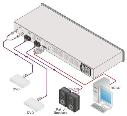
Figure 2: Connecting the 905xl Power Amplifier
