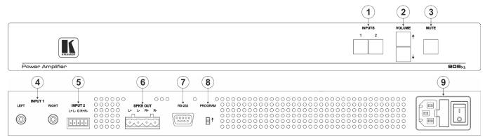
Figure 1 defines the front and rear panels of the 905xl.
