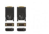
The 614T and 614R are a small and lightweight, detachable optical transmitter and receiver pair. They transmit uncompressed DVI resolutions of up to 1920x1200 at 60Hz using one multimode fiber optic cable with SC connectors. The 614T converts the DVI signal to an optical signal that it transmits to the 614R. The 614R decodes the optical signals back to a DVI signal
